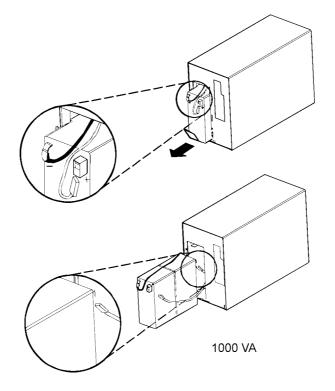
4. 1500 and 2200 VA units. Pull the battery out onto a flat, stable surface. Press on the black tab on the battery cable connector to disconnect the battery. See "Recycling the Used Battery" on page 20 for proper disposal.
